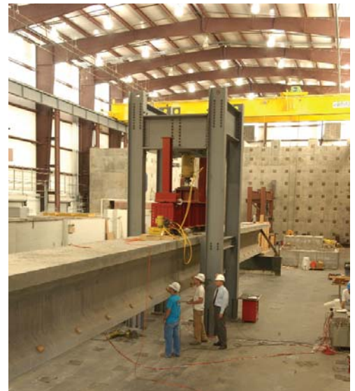
Full scale testing of lightweight high-strength bridge girder.
