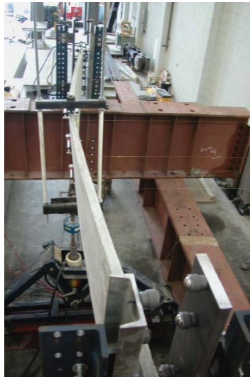
Lateral stability tests of reinforced and prestressed concrete beams.
