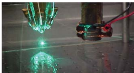
Fiber optic laser interferometer for structural damage detection.
