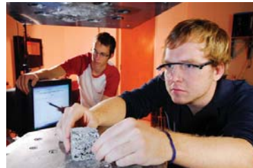
Students prepare test samples of Cenocell, a new material made from coal ash.
